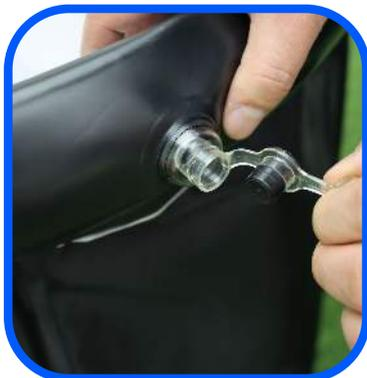
Once fully inflated, seal the top ring valve with the safety cap.
